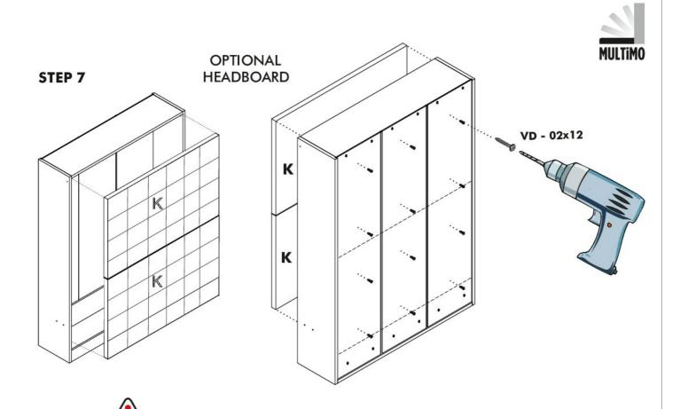
Must be secured to the wall made of brick, concrete or similarly strong material.
